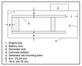
Figure 3-1 Mounting Surface Detail
